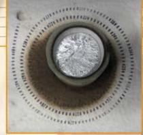
The measuring scale gives a quick and accurate answer on the metal quaity.
